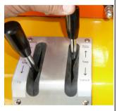
**TILT FORWARD OR VERTICAL** - The vacuum head can be tilted forward or vertically by pushing up or down the right lever on the control panel while depressing the green PUMP button.
