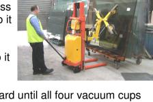
APPLY and move the Horizon forward until all four vacuum cups are on the glass. Once a safe level of vacuum is achieved the vacuum pump will turn off (you will hear the pump stop and notice the white vacuum pump light on the vacuum pump control panel switch off).
